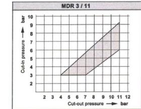
**Example:** Cut-out pressure p = 5 bar, cut-in pressure p<sub>e</sub> between 2,2 and 3,8 bar possible, all values can be adjusted in the grey field.
