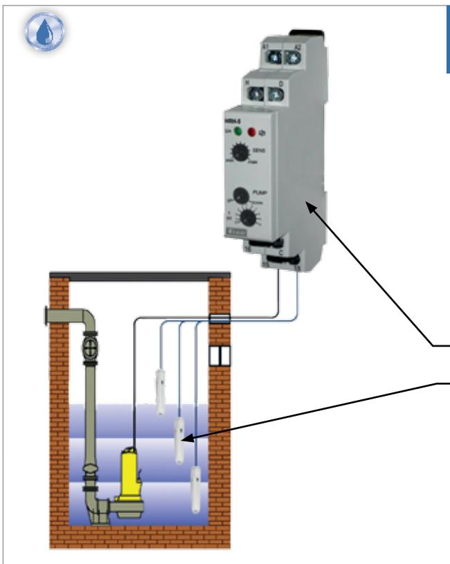
In this application, immersion electrodes are connected to an electronic analyser. When the electrodes are moistened by the liquid being measured, their conductivity alters correspondingly. One or two variable threshold values can then be adjusted.
