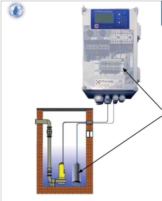
In this application, a level sensor is lowered into the medium within a sealed enclosure, whereby ceramic or piezoresistive sensors are used. The filling level pressure then acts directly on the ceramic or piezoresistive sensor and the subsequent value is then transmitted as a 4-20 mA signal via the connecting lead.
