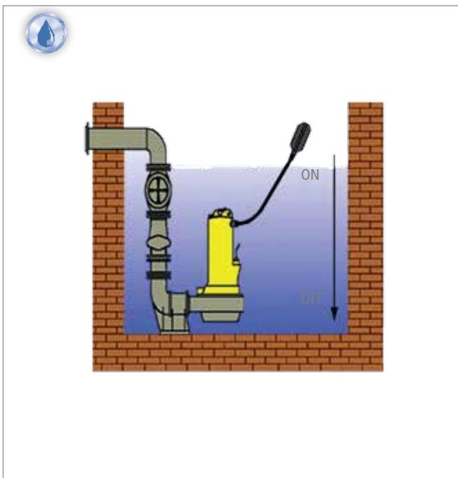
In this application, contacts placed within a floating enclosure are closed / opened depending on the inclination angle of the float switch.
