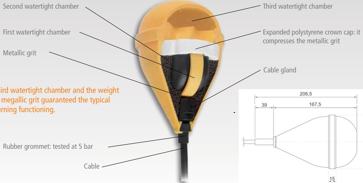
The third watertight chamber and the weight of the metallic grit guaranteed the typical overturning functioning.
