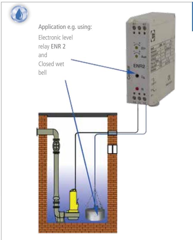
In this application the level change is transmitted via a pneumatic tube to the sensor and evaluated. The two types of systems - closed and open - are described in more detail below:
